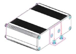
Mount the switch to the required surface using appropriate fixings
