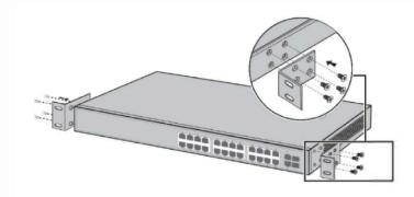
Once the brackets are securely fitted, the unit should be positioned so that the mounting holes in the brackets are aligned to the rack holes. The unit should then be secured using captive fixings, to ensure the device is secured in the rack assembly. Note — if you are using the rear GND terminal, then you may have to attach your Ground Cable before installing the unit into the rack, depending upon whether or not your rack has an open rear access panel or door.
