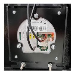
Connect the Duo Clasp connector to the socket located on the rear of your Nayax Unit. Here it is shown installed, but we recommend fitting this connector before installing the unit.
