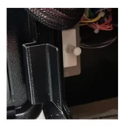
Tidy up the cable assembly harness by routing the Nayax Interface Cable through the mesh shield located above the door interlock switch
