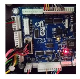
Apply power to the machine or activate the +48VDC by operating the interlock on the coin door switch, depending upon previous method of power isolation chosen earlier in the process
