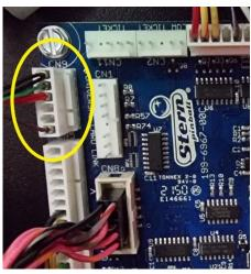
Ensure the machine power is switched off (or as a minimum, ensure that the +48VDC supply to the Cabinet Node Board is disabled by opening the coin door switch)
