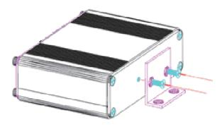
Attach the Wall Mount Bracket (if not fitted) to the switch case using the screws supplied
