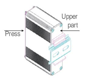
Clip the upper edge of the bracket onto the DIN Rail and push to latch the bottom strip
