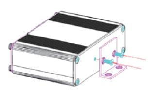
Attach the Wall Mount Bracket (if not fitted) to the switch case using the screws supplied
