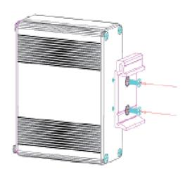
Attach the DIN Rail Bracket (if not fitted) to the switch case using the screws supplied
